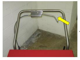
The 34 sweeper has a large lever to control the speed. The large lever makes it easy for all users to be able to grip it. It also serves as the brake control when pushed down.
