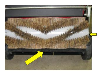
The 34 employs an attenuator flap, recycling flap and rear air control curtain. The attenuator flap keeps debris from cycling over the broom, while the recycling flap helps direct debris back into the broom. The air control curtain manages airflow from the back of the machine, and improves dust control.
