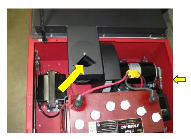
A feature to 34 sweeper is the Wet Sweep ByPass door. The operator can simply rotate this cover open to reduce the airflow into the filter when water on the ground is encountered.
