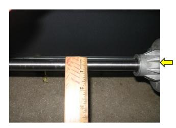
The 34 sweeper 1" axle is larger than axles on many other machines. The larger axle is designed to support the unit in harsh applications and last the life of the machine.
